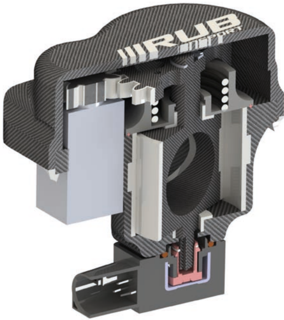
Hybrid throttle valve for a formula racing car
