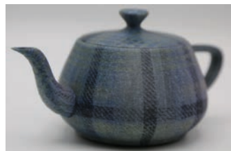
Figure 1: A 13-cm teapot printed with a dishcloth displacement map (left) and without (right). The fine-scale surface detail and visual realism costs less than 1MB in extra storage.
