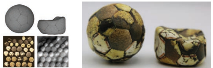
Input Print Figure 2: A model comprised of disjoint mesh patches, a displacement map, and a color texture map (left), and the resulting print using displaced signed distance fields (right). The total geometry storage is only 2MB.
